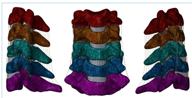
Figure 2. The three-dimensional finite-element model of C3-7.
